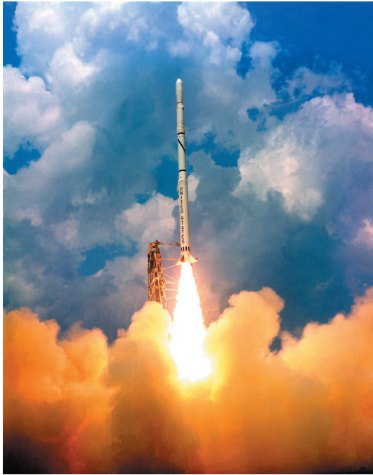
Four-stage, solid propellant Scout rocket.
