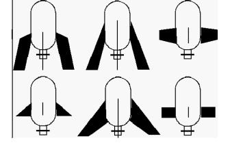
\*\*\* Spiral flight helps stabilize the rocket the same way a football is stabilized by spinning in flight. However, this spinning motion does tend to use up some of the energy needed for forward motion. To make a rocket spin, angle the fins slightly when attaching the fins to the rocket or bend the tips of the fins in a pinwheel fashion.
