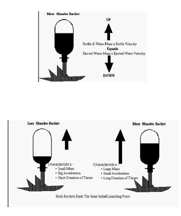
• Essentially, the faster the fluid is ejected, and the more mass that is ejected, the greater the reaction force on the rocket.
